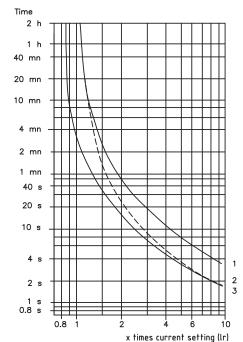
—— Balanced operation, 3-phase, from cold state.
