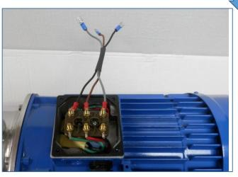
Connect the cable supplied to the motor terminals of the pump
