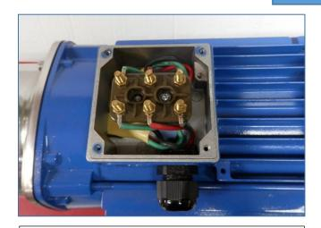
Open the terminal block case of the motor
