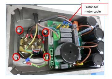
Opent the Speedboard, connect the earth cable of the pump to the faston of the Speedboard and fix the Speedboard to the pump with 4 screws directly to the case of the motor. Connect the faston of the motor cable to filter electronic circuit.
