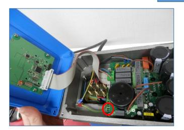
Connect the display cable, connect the pressure sensor cable on the terminal block indicated on the figure.
